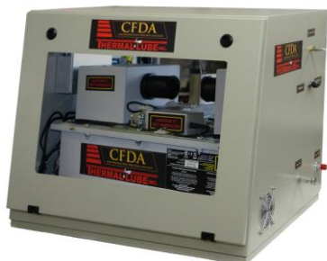
Figure 1. the CFDA system used on real-time monitoring of transesterification process.
